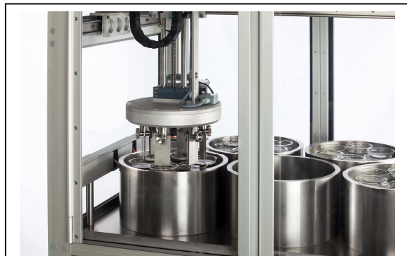
Picture 2: Detailed view of the test plates above the individual glass beakers.
