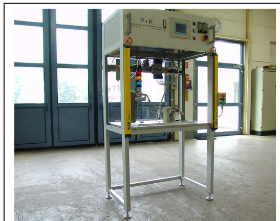
Fig. 1: Leak test bench for safety-related welded and bent components.
