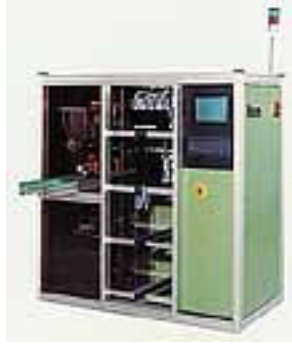
Fig. 4 Fully automatic in-process testing system for electrical equipment, linked to the conveyor system, interchangeable modules allow rapid change-over from one product line to the next. 1984 (Name of graphical metafile: Foto_3.tif)
